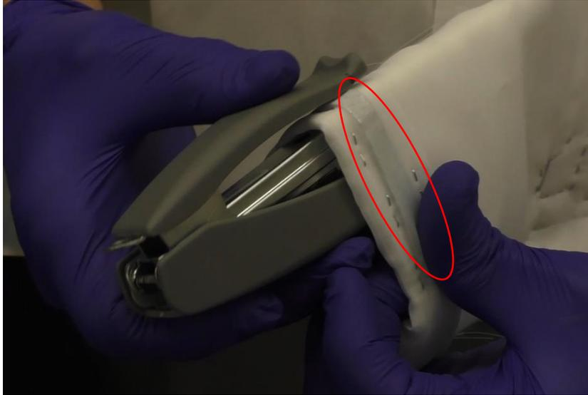
**Figure 9:** Metal nose-piece (circled in red) captured between layers of sheer material using parallel rows of staples along edge of filter stack.
