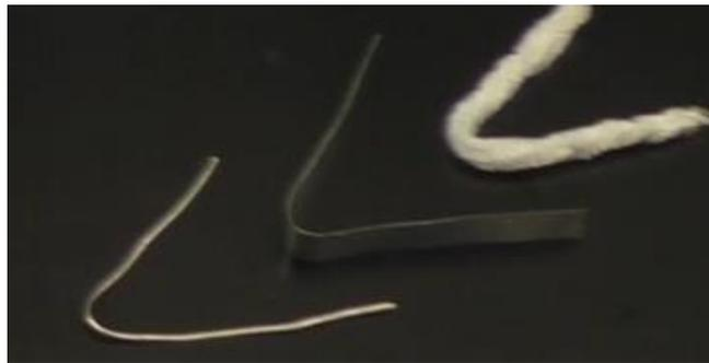
**Figure 4:** Final shape of malleable metal nose-piece to be created.
